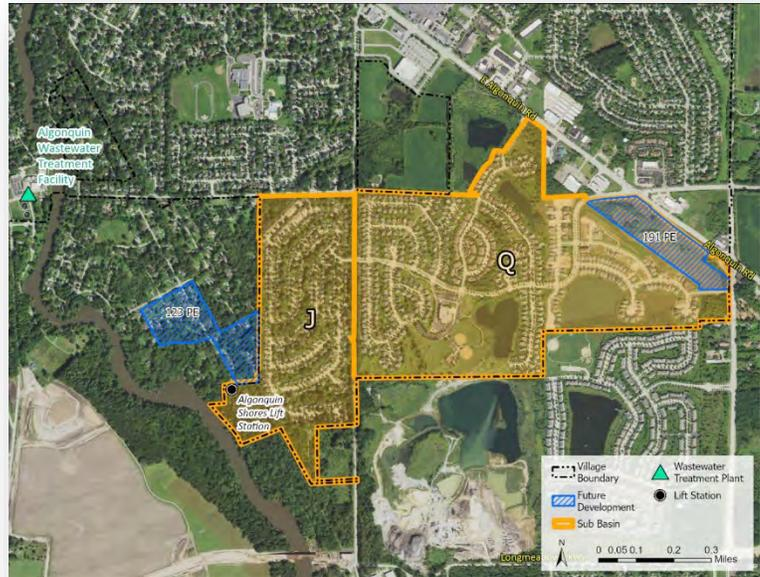
Wastewater is pumped through a 10-inch diameter, 3,300 lineal foot force main. Prior to 2024, the force main reduces from a 10” diameter pipe to 6” at the intersection of Riverwood Drive and Stratford Lane, creating a bottleneck in the system. In 2024, the bottleneck was removed and the existing 6” force main was replacement with 10” diameter pipe.
