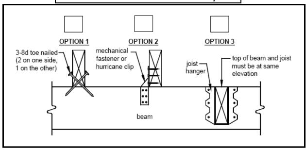
Please choose the appropriate beam configuration and joist-beam connection for your project. Please fill in all blanks.
