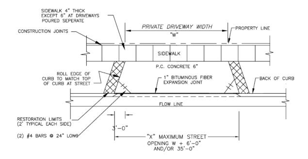
CONSTRUCTION JOINTS SHALL BE PLACED IN A UNIFORM MANNER THAT ALLOWS NO SINGLE SLAB BE MORE THAN 10 FOOT BY 10 FOOT DIMENSIONALLY
