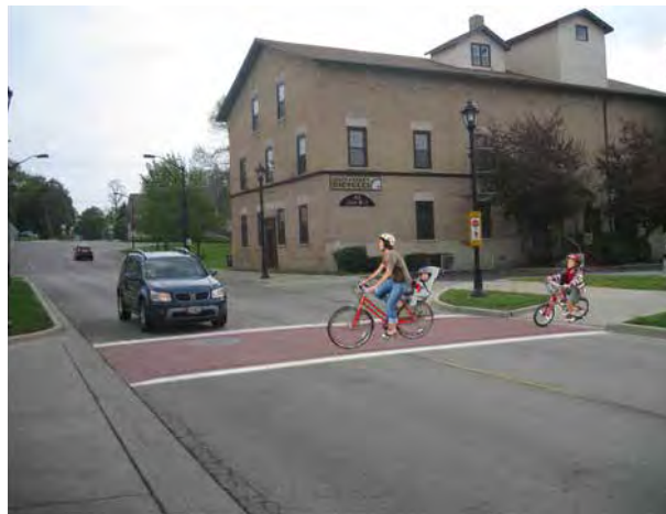
Illustration of an improved Fox River Trail crossing over Main Street in Old Town Carpentersville. Brick pavers and pedestrian-scaled lighting could improve the visibility of the crossing for both bicyclists and motorists. Source: Village of Carpentersville Old Town Plan, 2012, CMAP.
