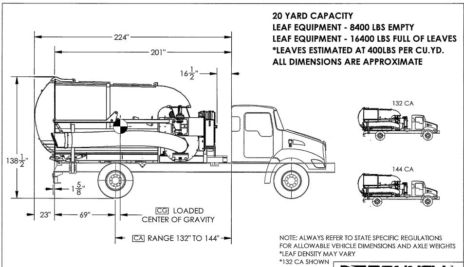
NOTE: RECOMMENDED AXLE RATINGS ONLY VALID IF NO OTHER EQUIPMENT IS INSTALLED ON TRUCK
