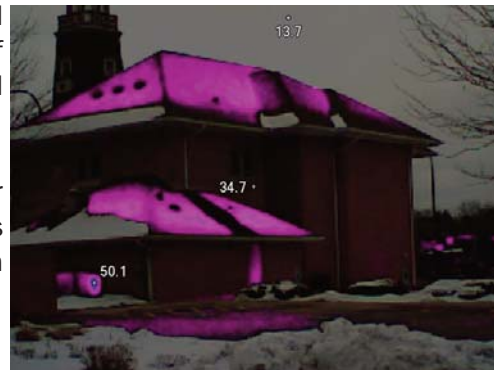
Thermal image of Historic Village Hall displaying heat loss through roof.
