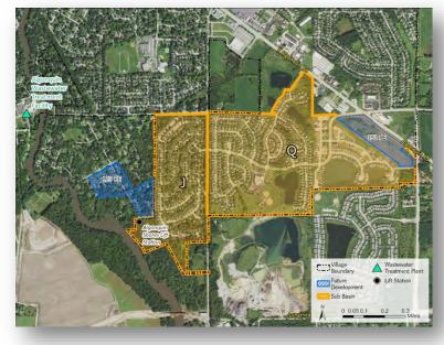
Wastewater is pumped through a 10-inch diameter, 3,300 lineal foot force main. Prior to 2024, the force main reduces from a 10" diameter pipe to 6" at the intersection of Riverwood Drive and Stratford Lane, creating a bottleneck in the system. In 2024, the bottleneck was removed and the existing 6" force main was replacement with 10" diameter pipe.
