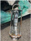
Description: old pneumatic post pounder, replaced with new hydraulic model.
