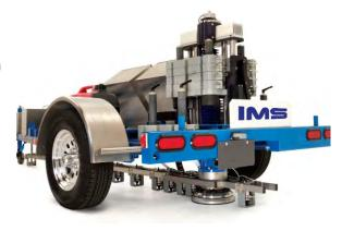
Fast Falling Weight Deflectometer (FastFWD)
