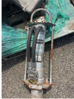
**Description: old pneumatic post pounder, replaced with new hydraulic model.**
